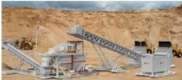
Mobile mining plant Makes sand into slurry/mud Pumps it to CDE sand plant
