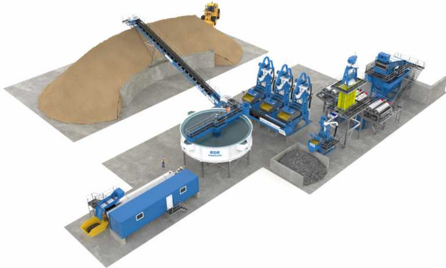
Example: Sand processing plant with magnetite recovery section
