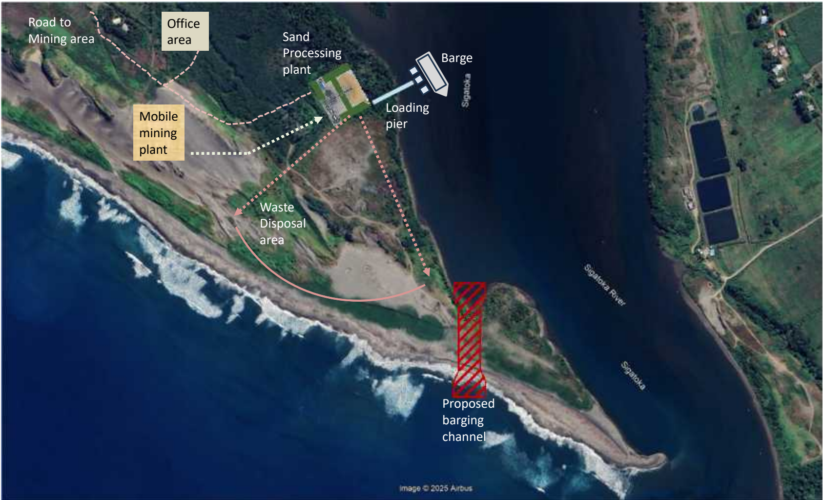
Proposed Position of all major mining, processing and support infrastructure equipment in Kulukulu South area
